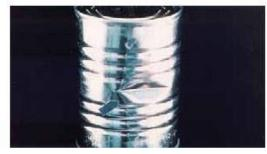
If the body dent does not significantly affect the side seam or double seams.
