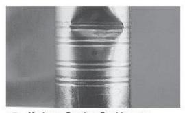
Moderate Denting. Double seam distorted, but not affected materially.
