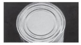
Ouble seam not severely damaged.
