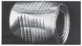
Paneled, beaded can. Materially affecting appearance, but not integrity, i.e. no plate fractures.
