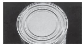
Ouble seam not severely damaged.
