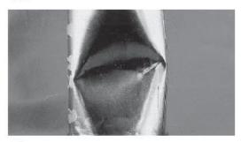
Severe body dent. Observe for fractured plate.
