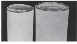
Gas formation in can which causes one or both ends to swell producing a flipper, soft swell, hard swell, or blown can. Hold for investigation.
