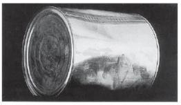
Paneled non-beaded can. Materially affecting appearance, but not integrity, no plate fractures.
