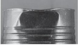
Severe body dent has affected double seam. Observe for fractured plate.
